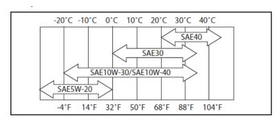
Using multi-grade oils (5W-20, 10W-30, and 10W-40) will increase oil consumption. Check oil level more frequently when using them.
