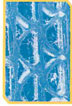
depth loading particles captured in filter
